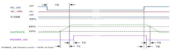
Above waveforms are expected with PS\_ON Signal ON/OFF state change:
